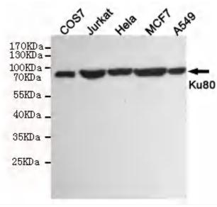
Western blot detection of Ku80 in COS7, Jurkat, Hela, MCF7 and A549 cell lysates using Ku80 mouse mAb (1:1000 diluted). Predicted band size:86KDa. Observed band size:86KDa.
